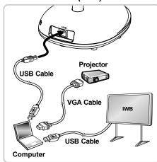
⚠ Once the USB is connected to the computer, the power is ON.
